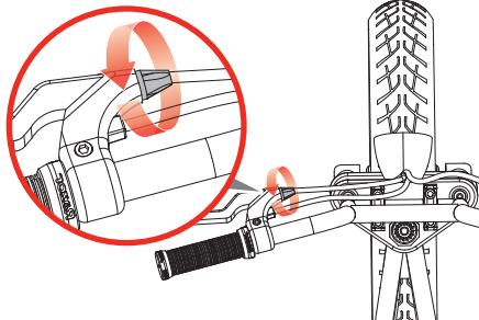
**EN** Loosen brakes at cable
